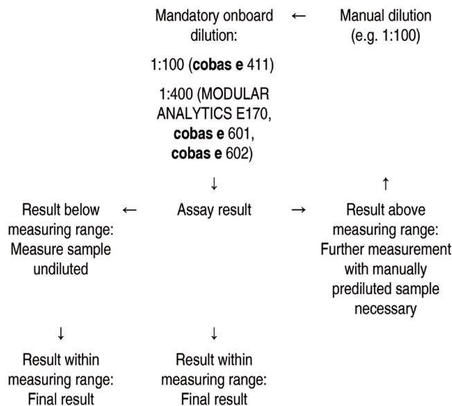
**Initial onboard dilution is mandatory for every sample.** Therefore every sample has to be run first with a dilution step ordered by the user and performed by the analyzer (1:100 on the **cobas e 411** analyzer and 1:400 on the MODULAR ANALYTICS E170, **cobas e 601** and **cobas e 602** analyzers).
